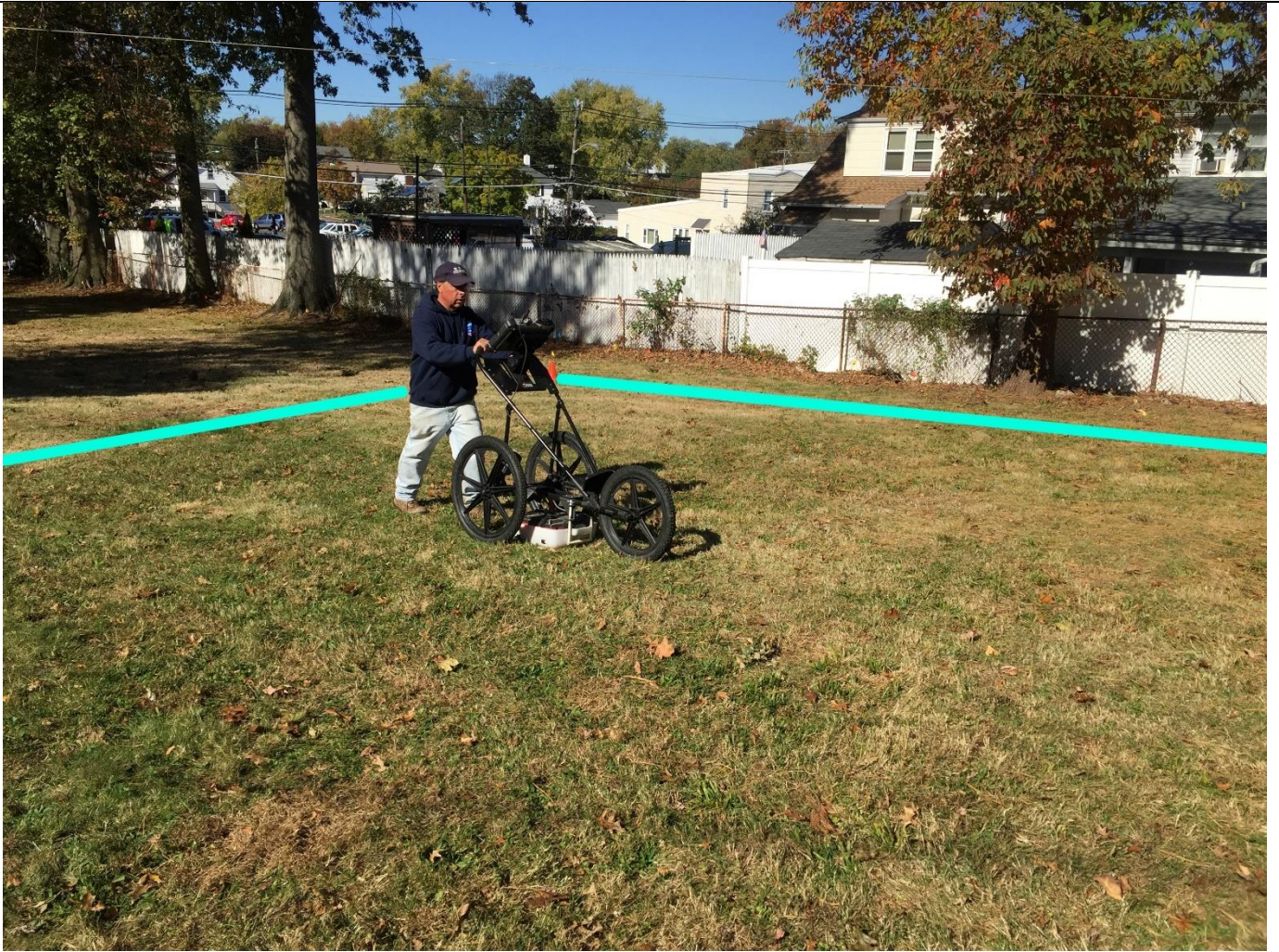
The 3D GPR Grid 1 survey being conducted within area of disturbance found during 2D survey. A portion of the 3D survey grid is outlined in aqua. View northwest.
